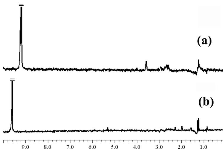
**Figure 7.** 1D-TOCSY spectra of the fresh *Mandanicese 2009* sample in  $\text{CDCl}_3$  with the selective excitation of the resonances at 9.18 (a) and 9.58 ppm (b). All the non-excitation signals are very weak and not assigned with certainty so far.
