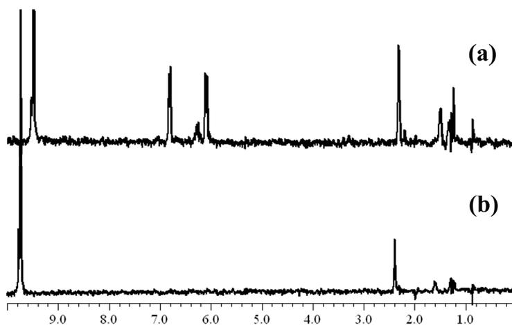
**Figure 6.** 1D-TOCSY spectra after drastic heating of the *Mandanicese 2009* sample in  $\text{CDCl}_3$  with the selective excitation of the resonances at 9.45 (a) and 9.71 ppm (b). Comparison with the TOCSY spectra of pure standards shows that these compounds are 2-E-hexenal and hexanal, respectively.
