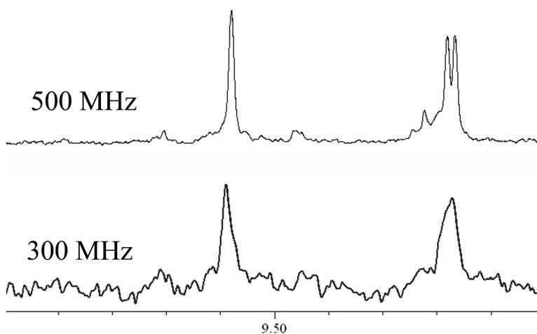
**Figure 3.** Expansion of the 9 – 10 ppm region of the DPGSE- $^1\text{H}$  NMR spectra run respectively at 300 and 500 MHz. Spectra were acquired with 64 transients in about 10 minutes.
