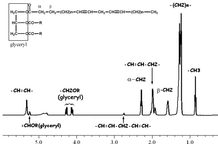
**Figure 1.** Main signal assignment in a  $^1\text{H}$  spectrum of the *Arbequina 2009* olive oil.
