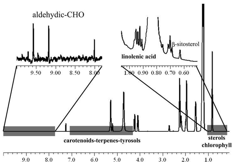
**Figure 2.** Selected expanded regions highlighting the presence of quantifiable species even just in traces. Reliable integration of the aldehydic region of a normal  $^1\text{H}$  NMR spectrum requires about 4000 transients and about 4 hours of experimental time.
