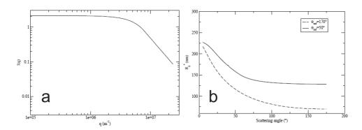
**Figure 1.** Calculation of  $R_g^*$  functions from the scattering angular signal. (a) Theoritical measurement of angular scattering and (b) Theoritical  $R_g^*$  for two  $\theta_{ref}$ .
