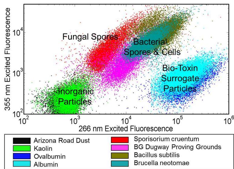
**Figure 1.** An illustration of the separation observed in measured UV-LIF emission intensities in two spectral channels from lab-generated populations of aerosol particles representing four broad groups: inorganic ambient background particles, fungal spores, bacterial particles (spores or cells) and bio-toxin surrogates (proteins). The eight specific example compositions are color-coded in the legend.
