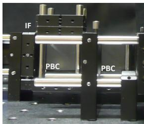
**Figure 1.** Photography of the novel home-built UV-polarization sensitive detector. Only the perpendicular channel is represented. PBC stands for polarizing beam-splitter cubes and IF for interference filter ( $\Delta\lambda = 0.35$  nm).
