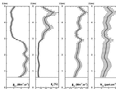
**Figure 3.** Vertical profiles of  $\beta_{p,||}$ ,  $\delta_p$ , backscattering coefficient  $\beta_{ns}$  and number concentration  $N_{ns}$  for non spherical (ns) ash particles on April 19<sup>th</sup> at 18h30.
