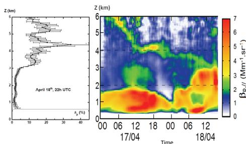
**Figure 2.** Vertical profile of the particle UV-depolarization ratio  $\delta_p$  and time-altitude map of the parallel particle UV-backscattering coefficient  $\beta_{p,\parallel}$  (color plot), showing the volcanic cloud in a filament tilting into the low troposphere.
