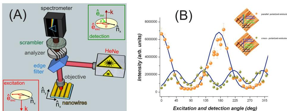
**Figure 1.** (A) Schematics of the experiment. Measurements are carried out in backscattering. The excitation polarization is varied by turning the sample underneath. The polarization analysis of the SERS radiation is carried out with a rotating Polaroid sheet. (B) Experimental behaviour of the parallel- (orange symbols) and of the cross-polarized (green symbols) components of the SERS emission. The blue lines are fits according to the theoretical model.
