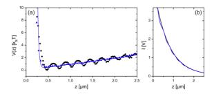
**Figure 2.** (a) TIRM with a reflecting particle (400 nm radius titanium-oxide particle [16]) and large penetration depth ( $\beta = 720$  nm). Under such conditions an exponential cannot be assumed and, indeed, the potential obtained the exponential I(z) is faulty (black circles). Using the fitted I(z) the correct shape of the potential is retrieved, with a short-range electrostatic repulsion and a gravitational slope far from the surface. (b) Exponential (black) and fitted (blue) I(z).
