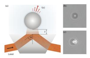
**Figure 1.** (a) Schematic representation of the TIRM working principle. The incoming laser is totally internally reflected at the glass-water interface generating an evanescent wave. A nearby colloidal particle scatters the light from the evanescent wave. The scattering intensity I(z) depends on the distance z from the colloid to the surface. (b) 4.3  $\mu$ m diameter polystyrene spherical particle illuminated in bright-field and (b) scattering of an evanescent wave.
