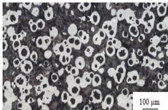
Fig. 2. Characteristic microstructure of the studied NCI, etched with 3 % Nital
