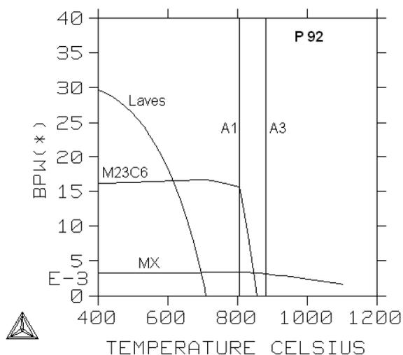
Fig. 2. Temperature dependence of weight fraction of minor phases in the steel P92 (ThermoCalc)
