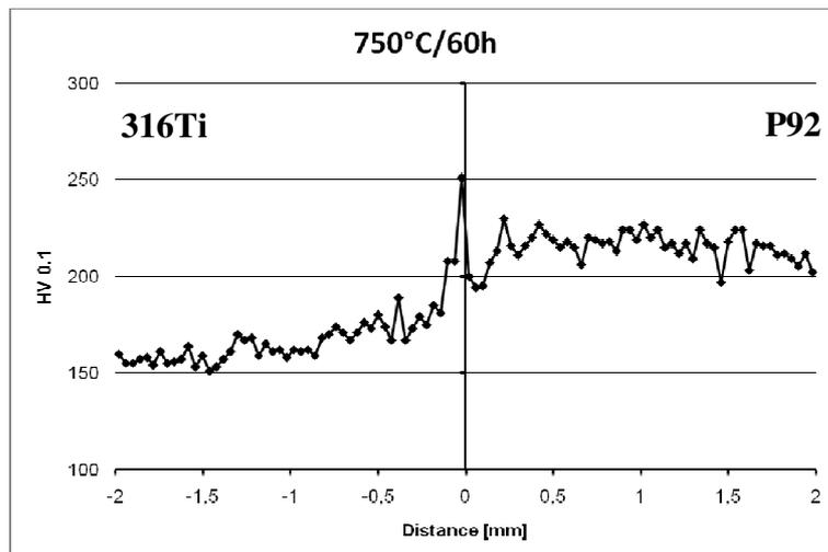
Fig. 6. Microhardnes values profile across the weld interface measured after annealing at 750°C/60h.
