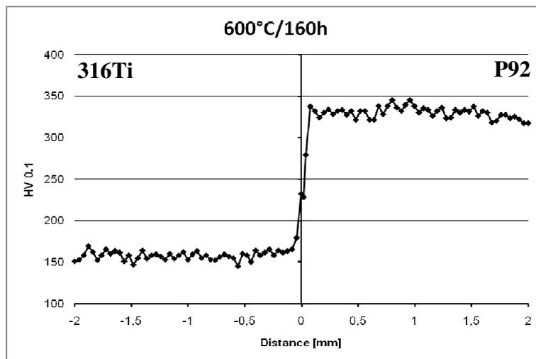
Fig. 5. Microhardnes values profile across the weld interface measured after annealing at 600°C/160h.
