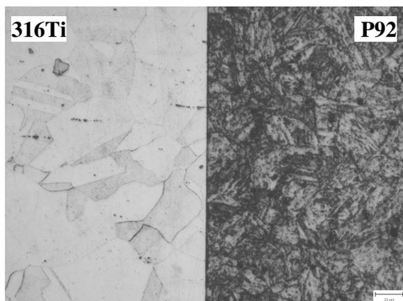
Fig. 3. Weld interface after annealing at 600°C/160h
