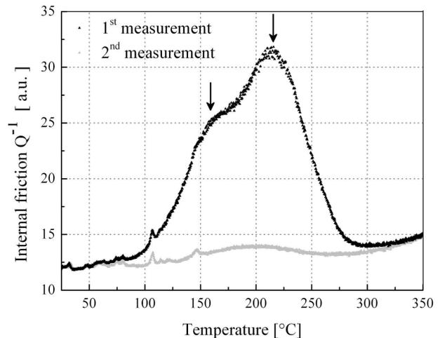
Fig. 4. Calibration measurements of IF on steel 12014
