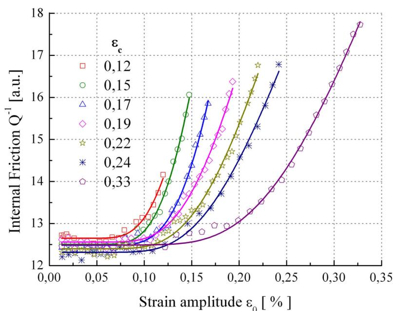
Fig. 5. Amplitude dependent IF measured on AZ31 at the temperature  $-15^{\circ}\text{C}$  after cycling at strain amplitude  $\varepsilon_c$ . Symbols represent measured data, lines comes from Granato-Lücke fit. (full colour version available online)
