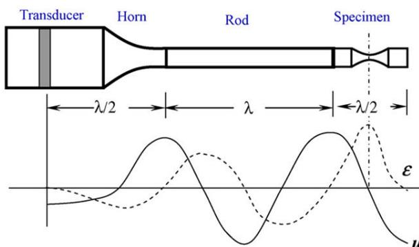
Fig. 1. Ultrasonic testing system[3]
