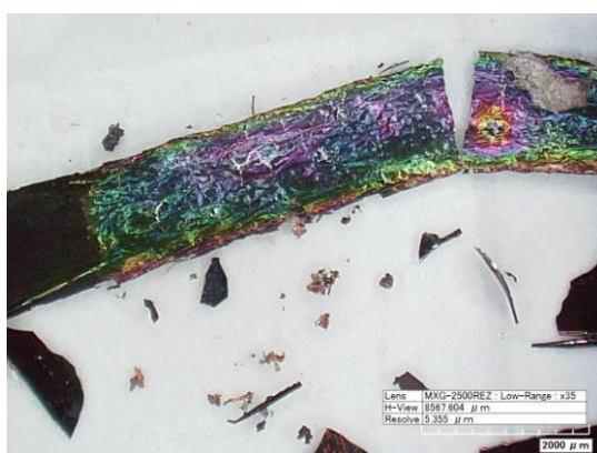
Fig. 10. "Active spots" on ribbon surface – \text{Mg}_{77}\text{Ni}_{17}\text{Pd}_3\text{V}_3 hydrogenated at 200 °C (a), hydride formation in active spots opens up surface layer – \text{Mg}_{87}\text{Ni}_{10}\text{Pd}_3 hydrogenated at 200 °C (b) (full colour version available online)
