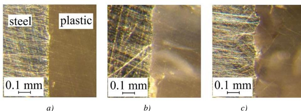
Fig. 16. Cross sectional view of bonds on the lateral surface.
