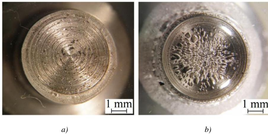
Fig. 8. Bubble formation at heating times of 3 s (a) and 7 s (b)
