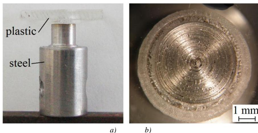
Fig. 2. The photo of the laser assisted hybrid joint, (a) side view, (b) top view
