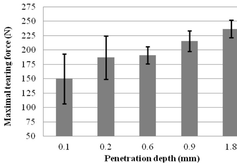
Fig. 7. Effect of penetration on tearing force
