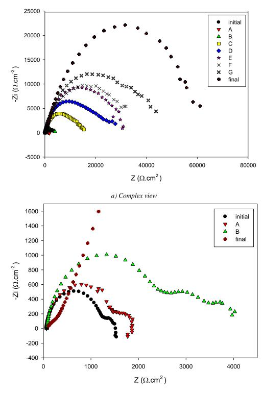
b) Detail Fig. 6. Nyquist plots of formed surface layer on AZ31 alloy at different stages of DCPD electrodeposition (0.9% NaCl electrolyte) (full colour version available online)
