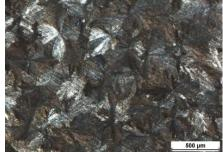
*i)* Final state (-0.012 mA.cm<sup>-2</sup>), t = 3000 s Fig. 5. Photodocumentation of calcium phosphate creation process by electrodeposition, light microscopy (full colour version available online)
