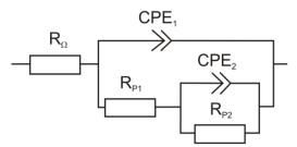
b) For Nyquist plots with two well-defined capacitive loops Fig. 2. Equivalent circuits used for analysis of Nyquist plots
