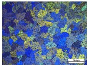
Fig. 1. Microstructure of AZ31 alloy, light microscopy (polarized light), etch. acetic acid + picric acid + water + ethanol (full colour version available online)
