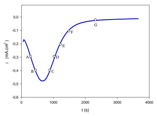
Fig. 4. Diagram of time dependence of current density during the electrodeposition process of DCPD (full colour version available online)
