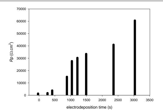
Fig. 7. Growth of polarization resistance during the electrodeposition process
