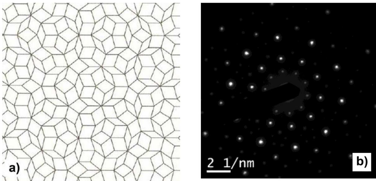
Fig. 1. a) Penrose tiling, b) diffraction pattern of Al-Cr-Fe quasicrystalline phase [1]
