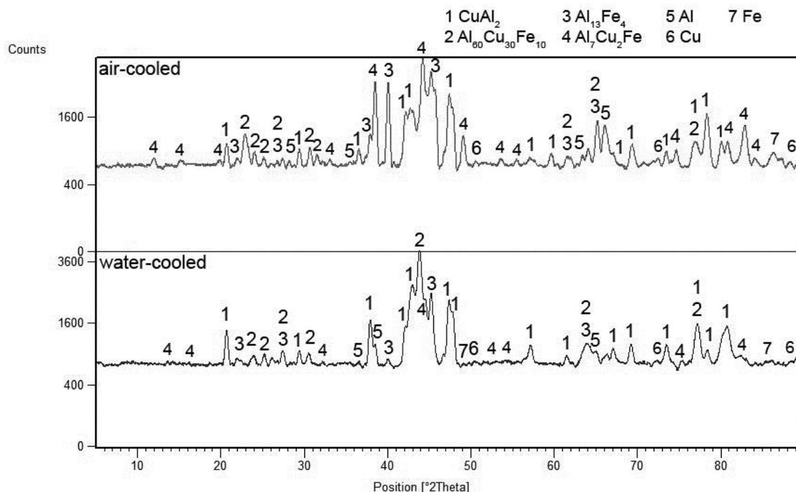
Fig. 2. XRD patterns of Al-Cu-Fe alloy prepared by SHS process followed by air cooling and water cooling
