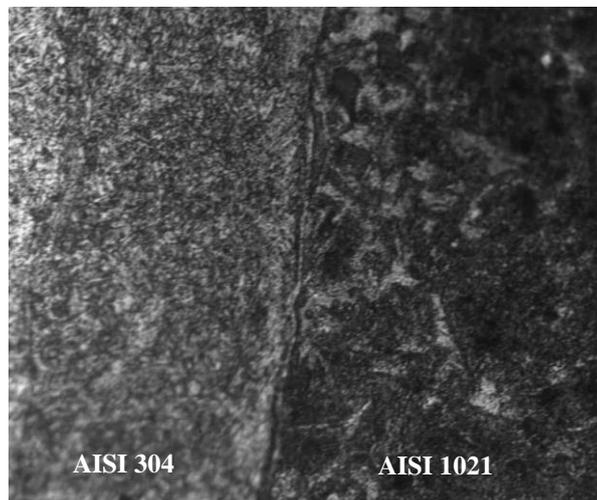
c) Optical microstructure of the joint
