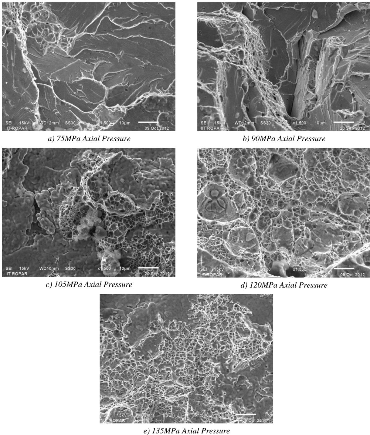
Fig. 3. SEM images at fractured interface during tensile testing.
