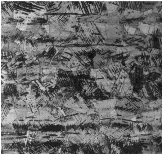
a) Optical microstructure AISI 304, etch. Ferric Chloride and Hydrochloric Acid
