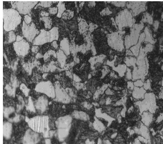
b) Optical microstructure AISI 1021, etch. Nital
