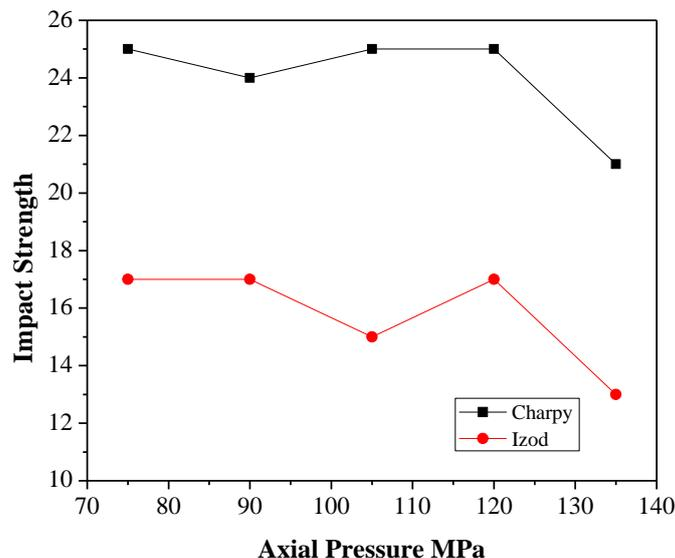
Fig. 4. Impact strength vs. Axial Pressure at 1000 rpm
