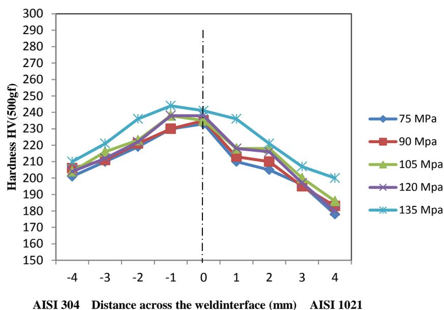
Fig. 5. Micro hardness at the weld interface.
