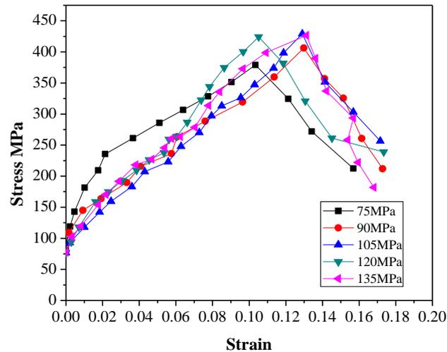
Fig. 2. Stress vs. Strain behavior of friction welded specimens at different axial pressures. (full colour version available online)
